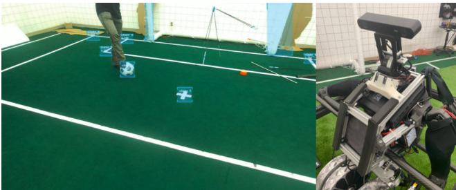
Figure 1. Object detection using YOLOv5 medium size (106 layers) to the left an photo of upper body and the neck of Artemis
